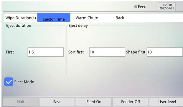
**Shape first (Eject delay)** : We separate Color sort and Shape sort Eject Delay time for better performance. When use shape arith, this value should be set according to material and machine model.
