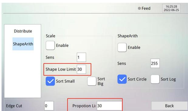
**Shape Low Limit:** For Scale arith use. Define the minimum material size, system will ignore materials smaller than this value.
