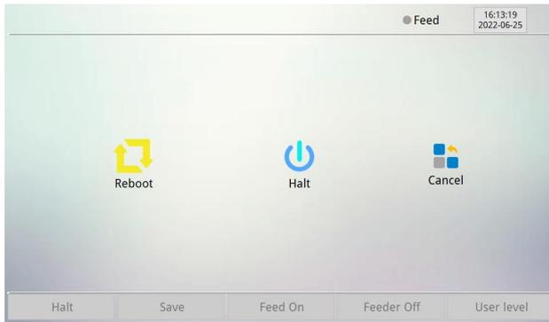
**Reboot:** Means reboot TS but not whole machine. Should notice that, Reboot won't automatically save parameters. Need to click "Save" button first.
