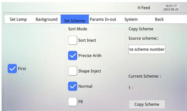
**Sort Inect**: For color sort arith use. Usually we disable this function. If this option is enabled, machine will reject any speckled or non-compliant material.
